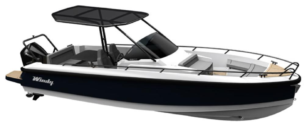
Length over all Beam 2,49 m Draft to prop 0,94 m Height (in storage) 2,2 m Dry Weight (incl. engine) Approx. 2 100 kg 300 ltr Fuel capacity
