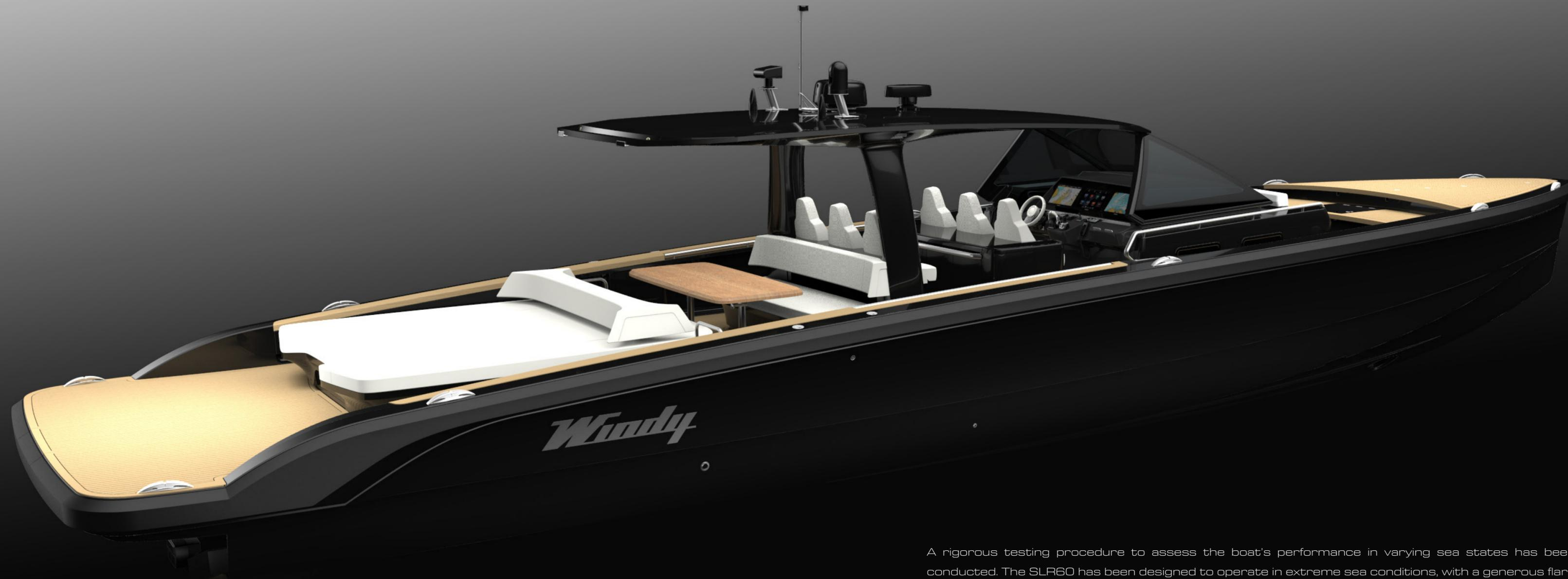
A rigorous testing procedure to assess the boat's performance in varying sea states has been conducted. The SLR60 has been designed to operate in extreme sea conditions, with a generous flare to the bow and multiple chines on the hull keeping the boat as dry as possible.
